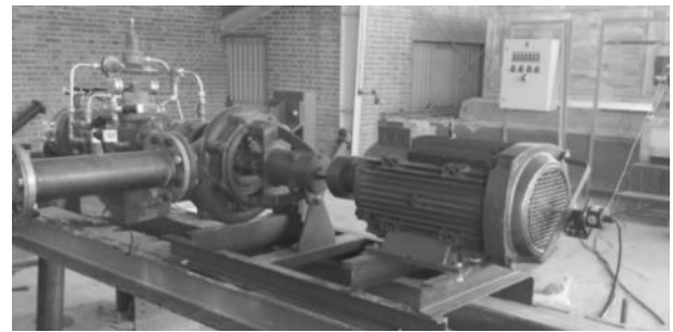
Fig. 10 Reverse pump in test circuit
