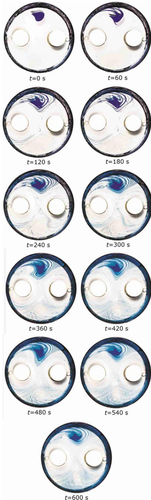
Fig 5 Dye mixing in the mixer with sinusoidal speed of rotors
