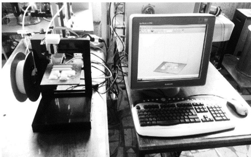
Fig. 1 UP! rapid prototyping machine while producing the measurement device mechanism parts
