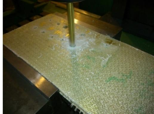
Fig. 4 3D composite during drilling
