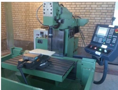
Fig. 5 CNC milling machine (FP4ME)
