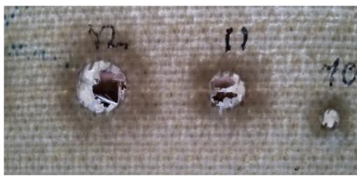
Fig. 6 Matrix fracture and uncut fiber in the hole
