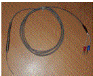
Fig. 8 K type thermocouple for measuring temperature
