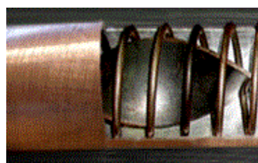
Fig. 7 The insertion of wire coil and twisted tape in the heat exchanger
