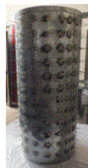
Fig. 4 Heated water storage tanks with installed fins
