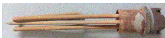
Fig. 5 Applied heaters for a basin solar still
