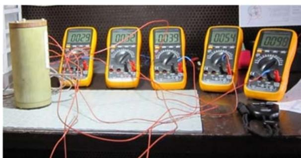
Fig. 4 Testing set up for powder thermal properties
