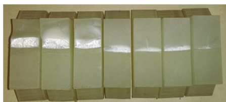
Fig. 16 Breaking open to expose of the crack surface after chilling specimens using immersion in liquid nitrogen
