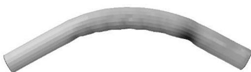
Fig. 9 Sample bending tube with wrinkling
