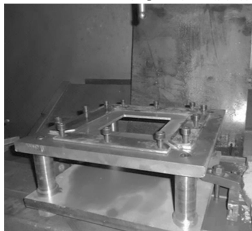
Fig.5 The experimental SPIF platform on the three axis CNC machine
