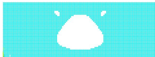
Fig. 9 The final topology of the stiffness-frequency reliability based topology optimization
