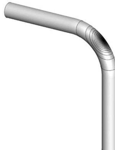
Fig. 5 Straight wire magnetic field distribution for unit of particle volume on bend are for case 1
