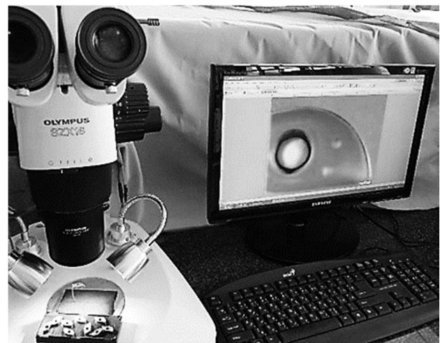
Fig. 3 Measuring setup of tool wear using SZX16 optical microscope
