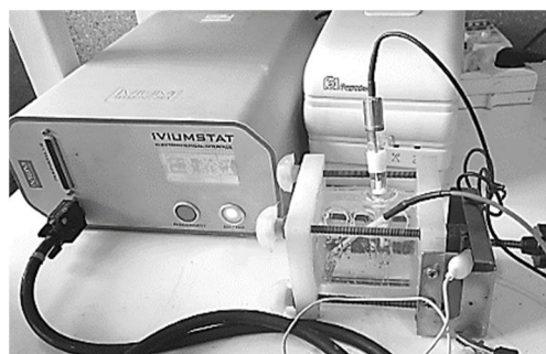
Fig. 5 Measuring method of electrochemical resistance of milled surfaces
