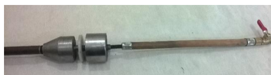
Fig. 10 Control valve connection to the main axle
