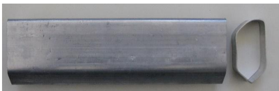
Fig. 19 The test result for tube filled with water at pressure equal to 6 bars using the three-piece die
