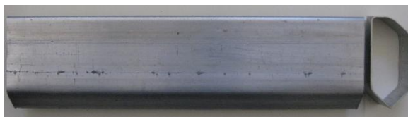
Fig. 23 The test result with hydraulic oil as the fluid using the three-piece die
