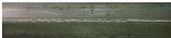
Fig. 24 Cracks appearing from sharp points in the final form
