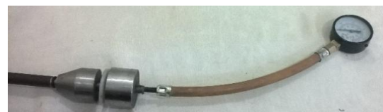
Fig. 9 Pressure gauge connection to the main axle
