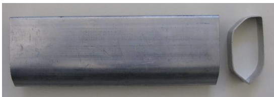
Fig. 20 The test result for tube filled with water at pressure equal to 7 bars in the three-piece die
