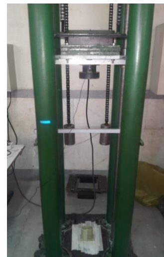
Fig. 2 Impact tests setup using Drop Tower machine
