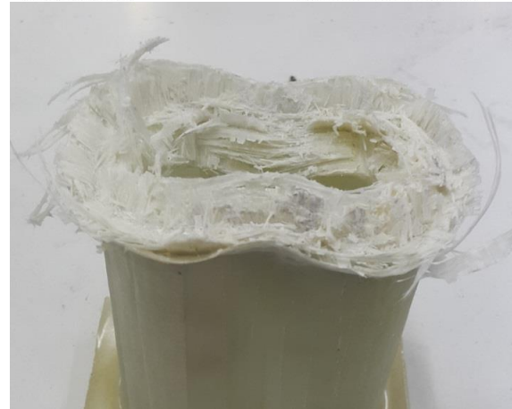
Fig. 11 Top and side view of crushed tubes under axial impact load
