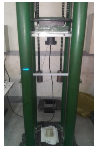
Fig. 2 Impact tests setup using Drop Tower machine
