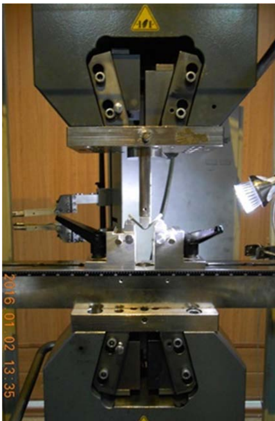
Fig. 8 The three-point bending test set-up.
