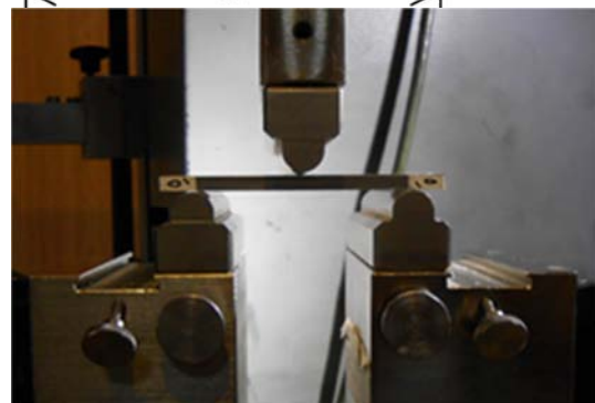
Fig. 6 Schematic and real view of fixture for the three-point bending test.
