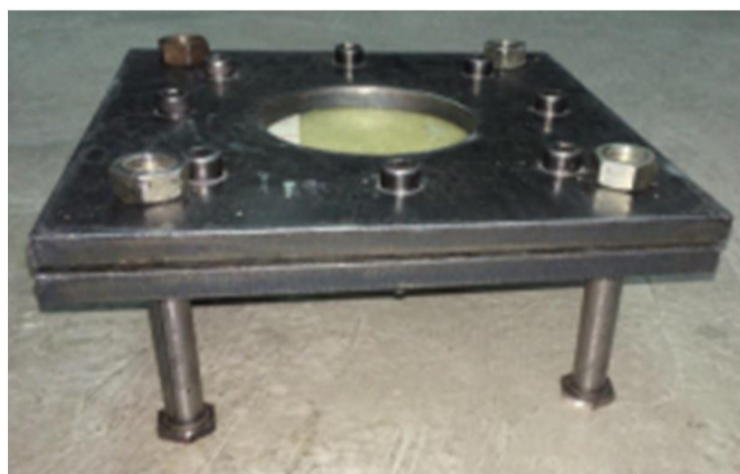
Fig.4 Fixture of punch shear for hybrid nanocomposite specimen
