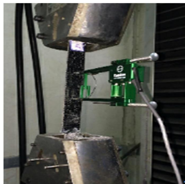
Fig. 5 Composite specimen under tension
