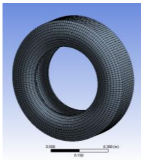
Fig. 8 Mesh of tire structural model
