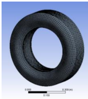
Fig. 9 Mesh of acoustic cavity model
