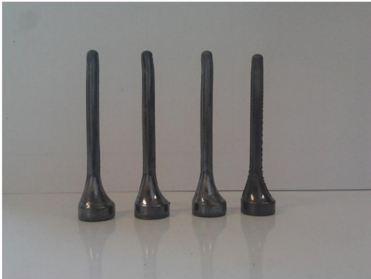
Fig. 12 Preform of successful extruded in die with temperatures 475, 450, 425, 400°C, from the left respectively
