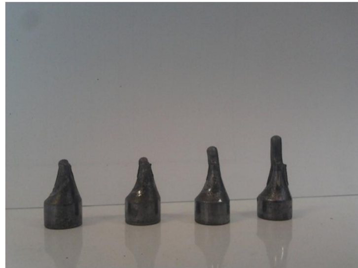
Fig. 13 unsuccessful preforms that produced in die with temperatures of 375, 400, 425, 500°C, from the left respectively.
