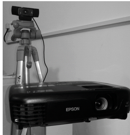
Fig. 6 used camera and video-projector as 3d scanner sensors
