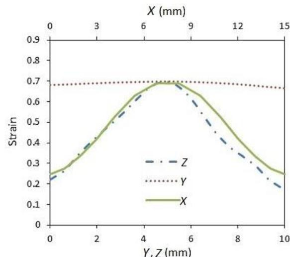
**Fig. 13** The distribution of the PEEQ resulted from the simulation along the  $x$ ,  $y$  and  $z$  axis
