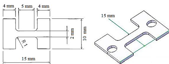
**Fig. 4** The schematic of the tensile test specimen designed in current research
