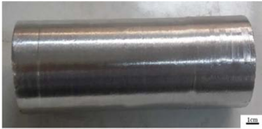
Fig. 3 Casting alloy sample after turning
