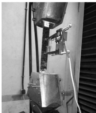
Fig. 3 The hybrid nanocomposite specimen under tensile test
