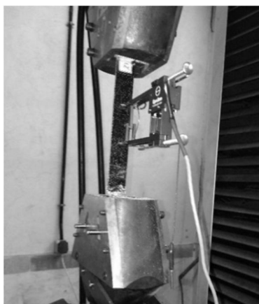
Fig. 3 The hybrid nanocomposite specimen under tensile test
