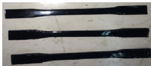
Fig.1 The tensile test specimens of the nano-resin
