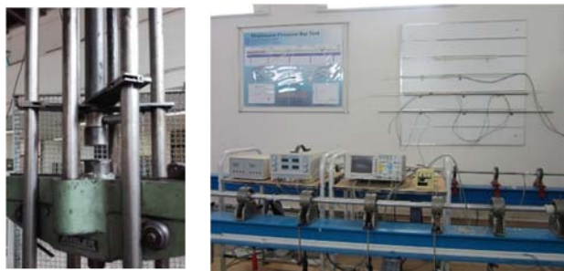
Fig. 5 Split Hopkinson Pressure Bar and Uniaxial Compression Tests
