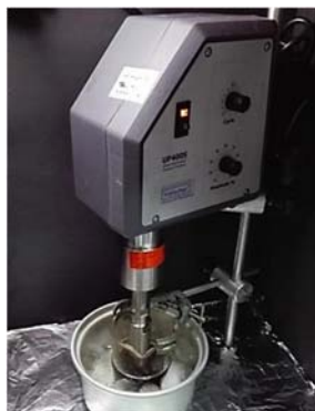
Fig. 2 Using of probe sonicator and ice bath
