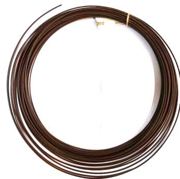
Fig. 3 FDM filament produced from ABS-Cu composite material
