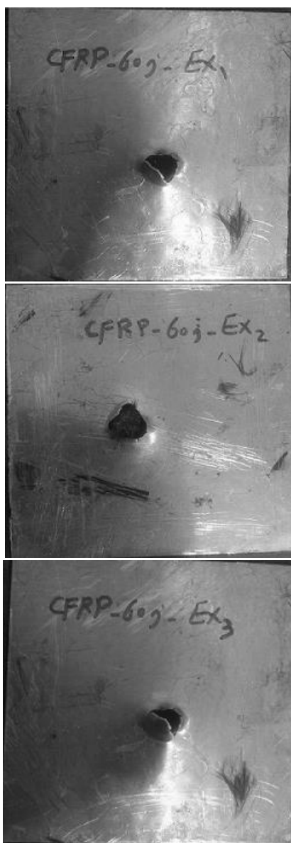
Fig.7 Comparison samples with 2-1 lay-up under 60j impact energy
