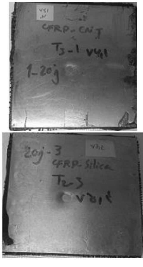
Fig.9 Aluminum front face damage a) with MWCNT b) with nano silica
