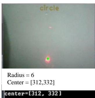
Fig. 11 Recognition of color, coordinates and radius of the laser light without obstacle
