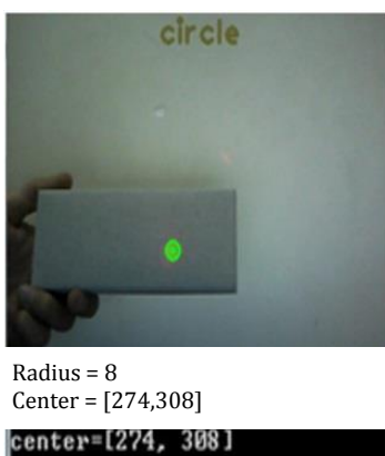
Fig. 12 Recognition of color, coordinates and radius of the laser light in the presence of obstacle
