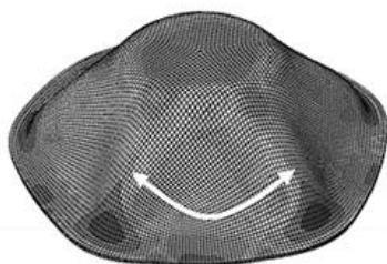
Fig. 7 Defined path on cone circumference for wrinkle wave study
