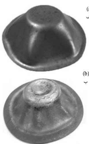
Fig. 11 a) Steel wrinkled conical cups b) Copper wrinkled conical cups, using HDDRP with inward flowing liquid
