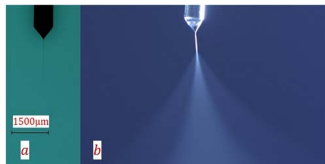
Fig. 13 Cone jet mode, (a): from shadowgraph, (b): from light scattering, Flowrate= 2 ml/h, Voltage= 4.63kV
