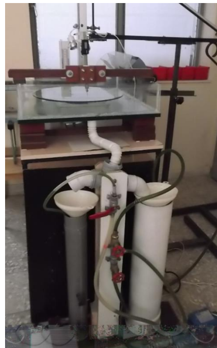
Fig. 2 The apparatus of the hydraulic jump in used for this work
