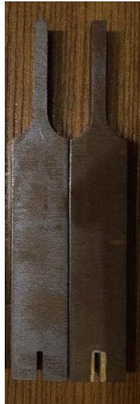
Fig.6 Fixtures made for fracture test
