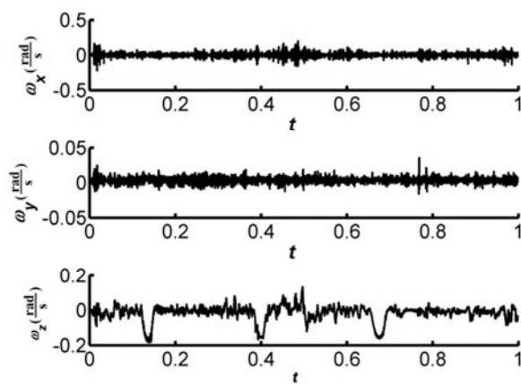
**Fig. 3** generated angular velocity signal in body coordinate
