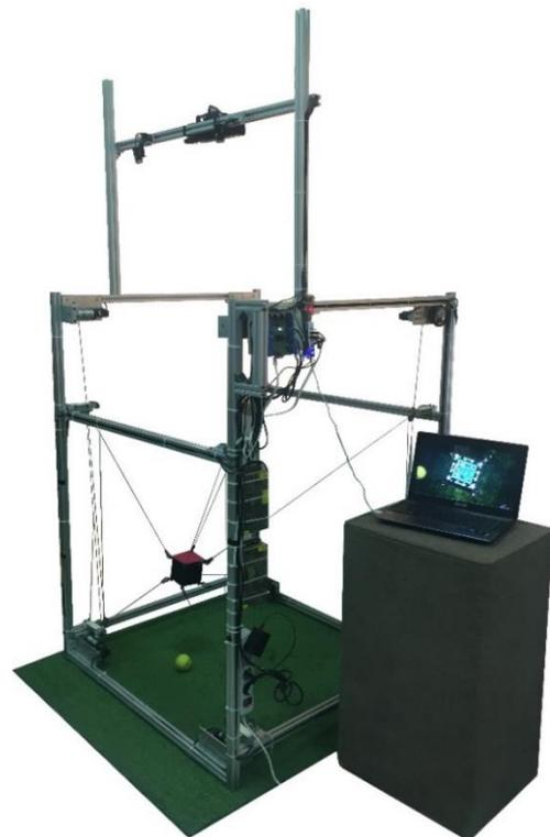
Fig. 1 6 DoF cable driven parallel robot, RoboCab
