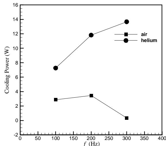
Fig. 11 Cooling power versus frequency,  $DR=5$ ,  $T_c=297$ ,
