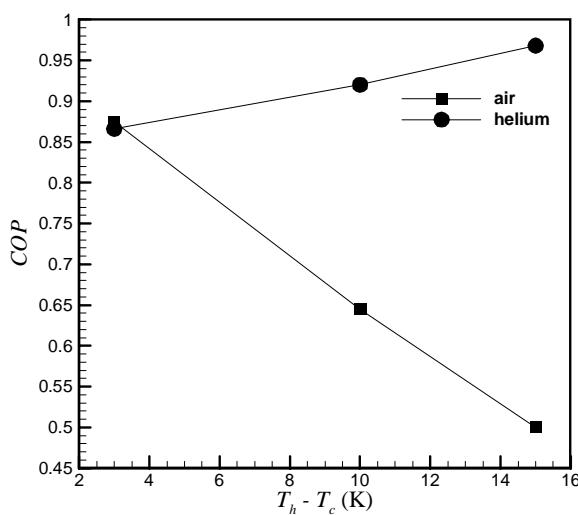
Fig. 9 COP versus heat exchangers temperature differencing,
