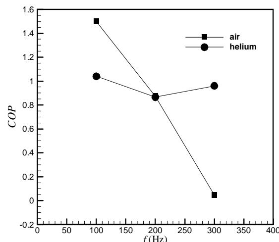
Fig. 12 COP versus frequency,  $DR=5$ ,  $T_c=297$ ,  $T_h=300$
