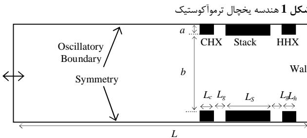
Fig. 2 Domain of simulation
