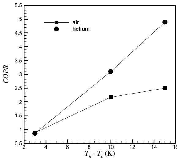
Fig. 10 COPR versus heat exchangers temperature differencing,
