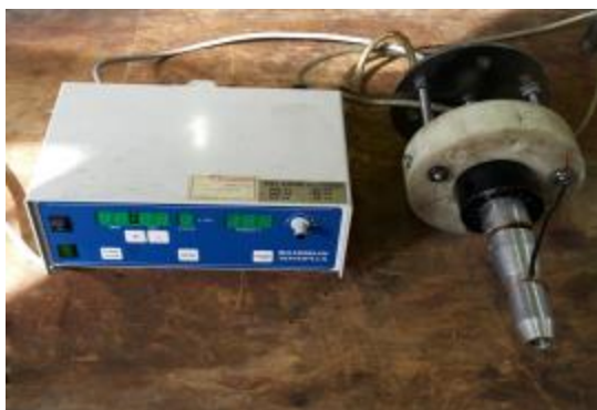
Fig.2 The ultrasonic vibration generator used for machining
