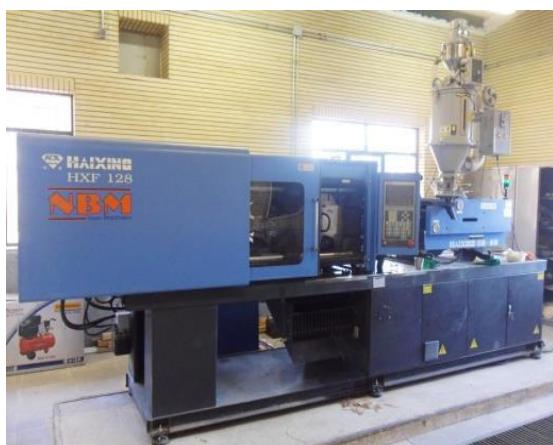
Fig. 1 Injection molding machine used in the research
