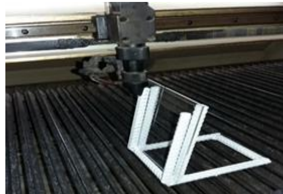
Fig. 3 Experimental determining of the focal plane position of the used CO 2 laser machine
