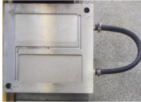
Fig. 2 used mold for producing the specimens
