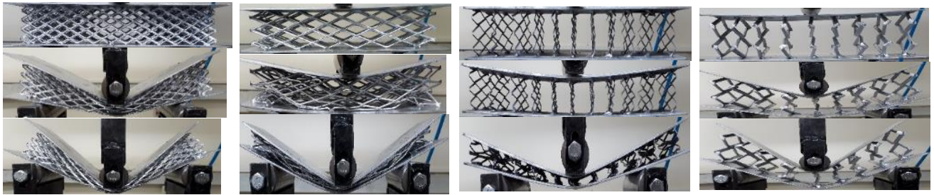
Fig. 16 a) A comparison of experimental force-displacement curves and collapse of the sandwich structures with lattice core b) BC3L2 c) BC2L2 d) BC262 e) BC162
