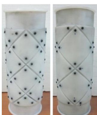
Fig. 1 The Polyethylene molds used for manufacturing the specimens
