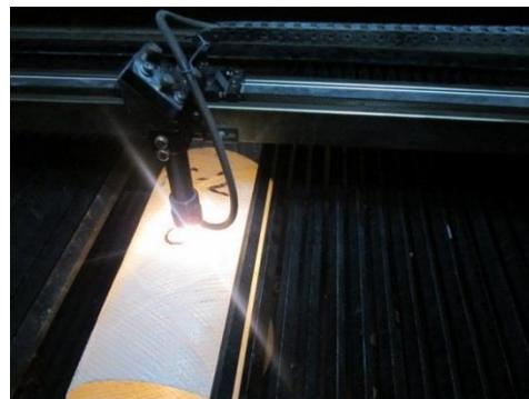
**Fig. 3** Create an opening on the shell
