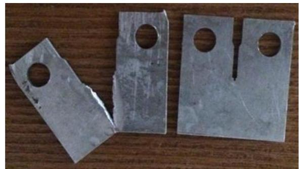
**Fig. 10** CT specimens before and after fracture test
