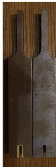
Fig.4 Fixtures made for fracture test
