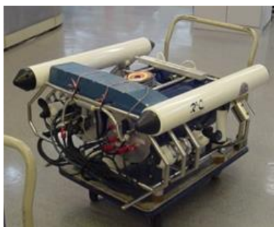
Fig. 2 RRC II underwater vehicle
