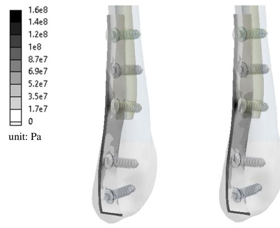
**Fig. 18** Stress at the plate under axial torsion load: a) First technique b) Second technique
