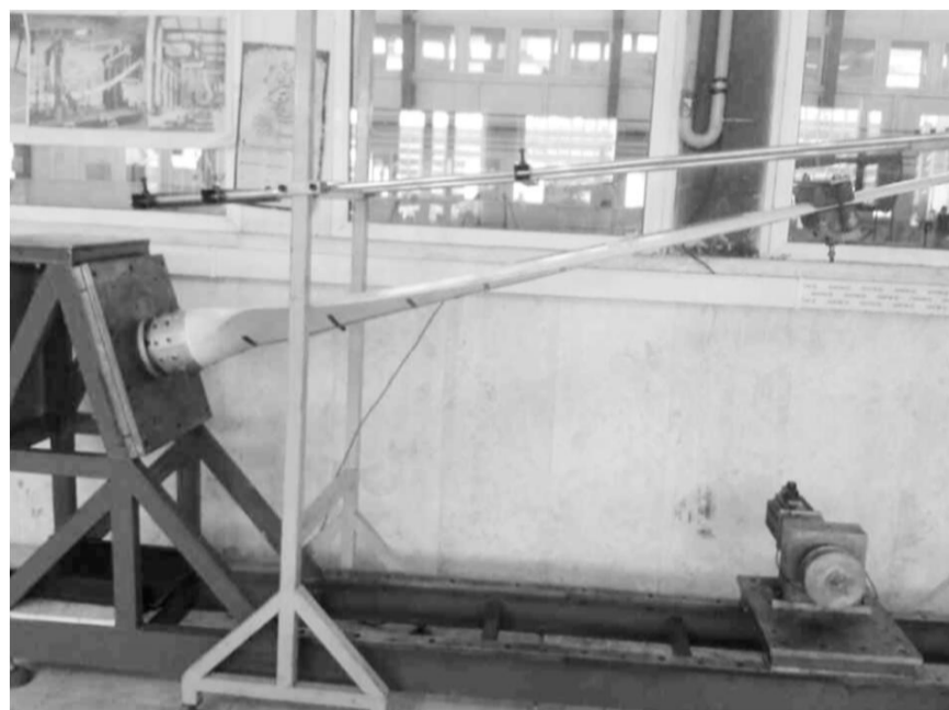
Fig. 4 Blade clamping structure
