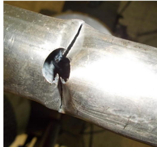
Fig.12 failure of specimen from location of cutout
