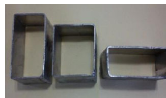
Fig. 2 Three manufactured Aluminum alloy samples with the same perimeter of quadrangular cross-section
