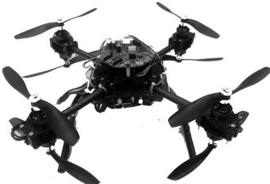
Fig. 13 Constructed Octorotor Flying Robot
