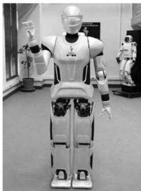
Fig. 1 SURENAIII humanoid robot
