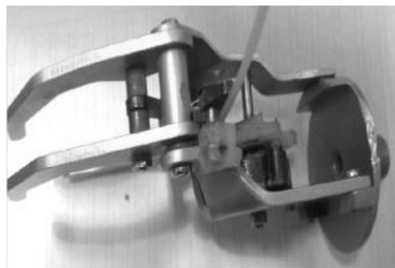
Fig. 2 Manufactured prosthetic hand model
