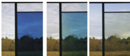
Fig. 2 The color change of electrochromic and thermochromic windows
